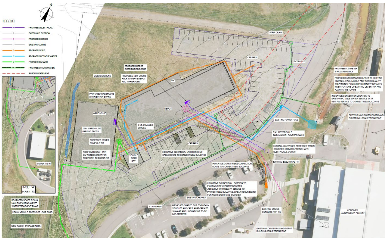
Figure 8 Utilities location and connection
