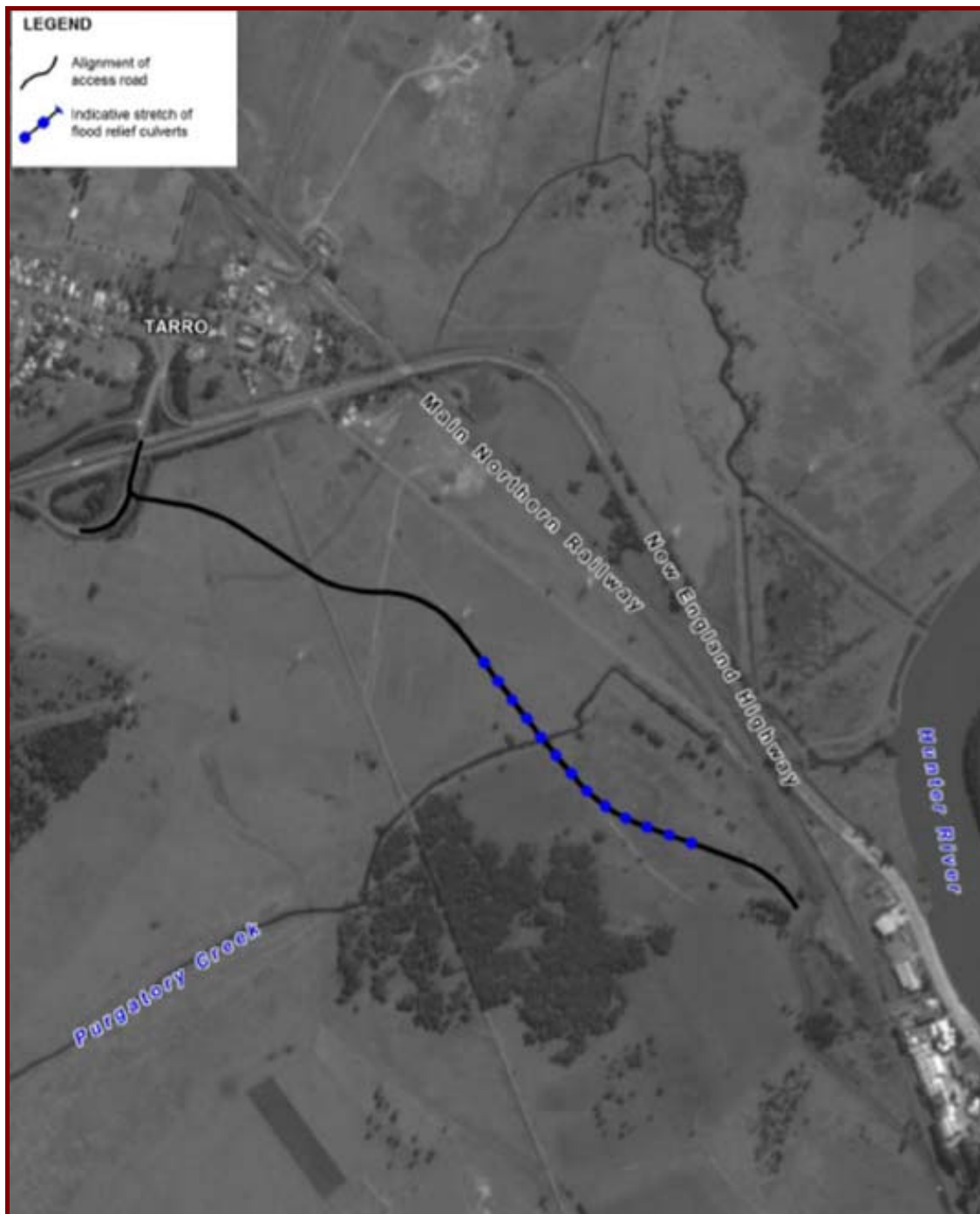
Figure 22: Location of Flood Relief Culverts Distribution.
